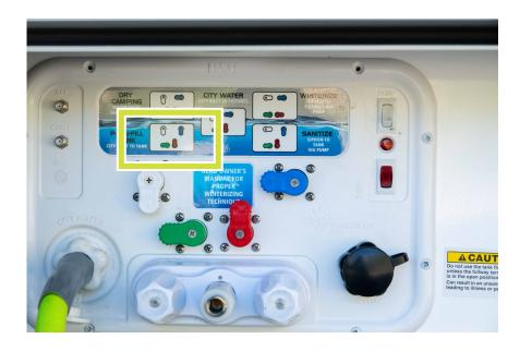
DO NOT OVERFILL THE FRESH WATER TANK. Monitor from the Center Panel inside the RV to ensure you do not overfill. You can disconnect the hose
