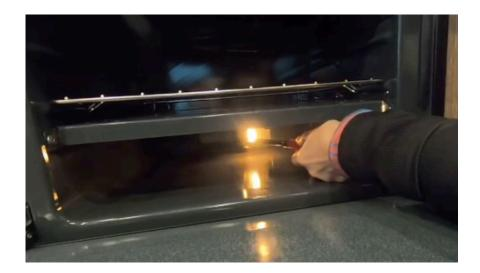
Once the pilot light is able to hold its own flame without the lighter present, you can turn the oven dial to the desired temperature. You should see the rest of the burner become lit as it warms up to the desired temperature.
