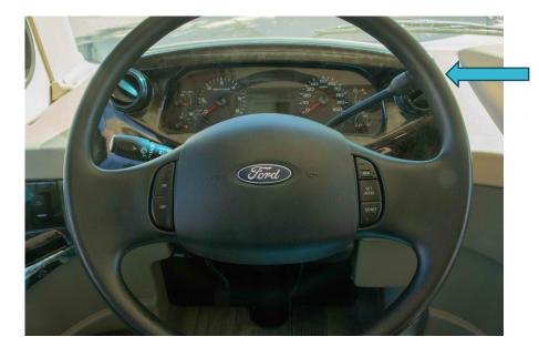
"Tow Haul" button at end of gear selector
