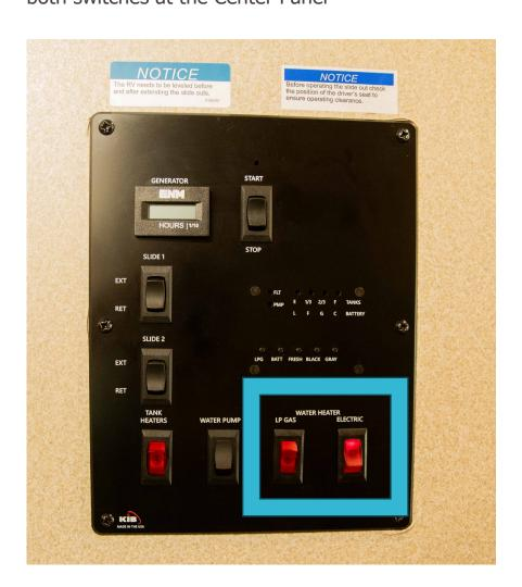
When not actively using the hot water, a good practice is to turn off the LP Gas and only use the electric to keep the temperature maintained. Then turn on the LP Gas when using lots of hot water (washing dishes or taking a shower).
