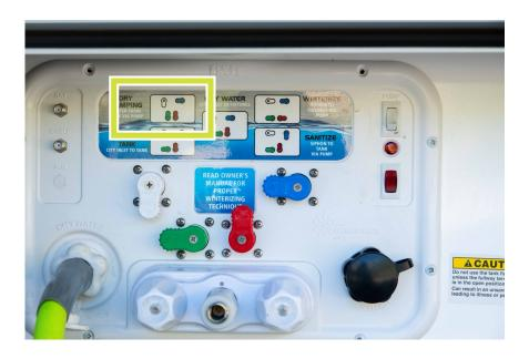
Then you will need to turn on the Water Pump when needing to run the water. You can do this from the Center Panel. Only run the water pump when you are actively using the water. Turn off the pump when not using the water to prevent the water pump from burning out.
