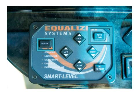
The Auto Leveling panel will blink "Excess slope" if it was unable to level due to a slope greater than what it can handle. If this occurs, either position the RV in a more level location, or you can place some yellow blocks underneath the pistons that were over extended (after you have retracted the pistons to reattempt). These blocks can be found in the furthest driver side rear compartment outside of the RV. Do not place more than four blocks underneath a piston.
